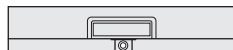
■ TUB-WALL RT 1 1200/200 200 x 1200 x 70 mm, with 1-sided slope, including loose sealing sleeve 370 x 1300 mm
