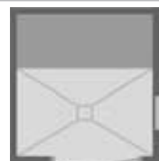
CAB-Q 1400 R.GR * door DIN right / bench seat opposite the door / installation wall right of the door
