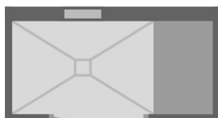
CAB-R 1780/950 L.RG * door DIN left / bench seat right of the door / installation wall opposite the door
